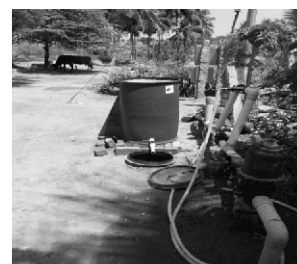
Ventury system used for fertigation of inputs
